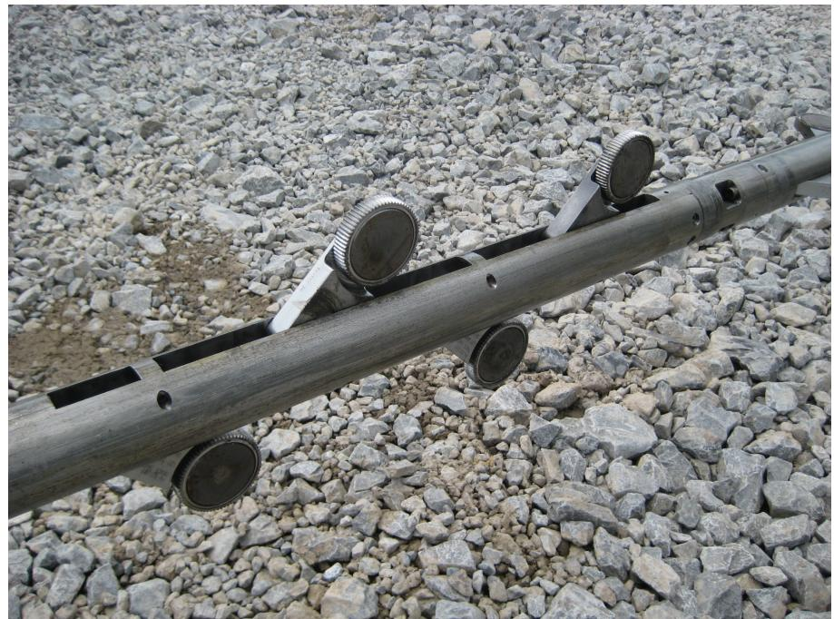
**Figure 7 – Wireline tractor tool used for deployment of logging tools in horizontal portion of Berea well.**
