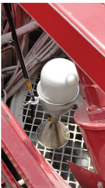
Figure 4 – Introduction of Boron Carbide during Frac Stage of Berea Sandstone well in Kentucky.
